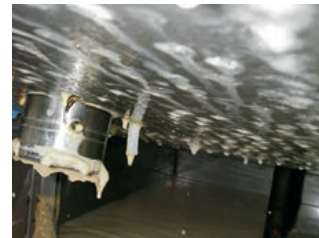
Biofilm formation on system cover which is a high recontamination source for fresh coolants
