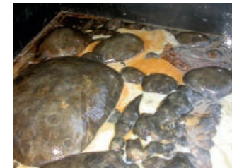
Extreme mould formation in contaminated system. In this case complete system sanitation with biocidal system cleaner and mechanical cleaning is crucial.
